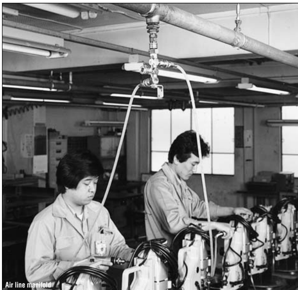
Air line manifold
