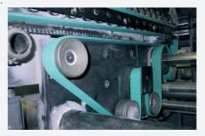
RAPPLON® folder and carrier belts give precise holding of the blanks throughout the entire process, whilst withstanding both mechanical stress and wear.
